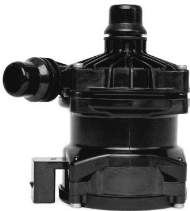
Fig. 2: Grivory HT1VA-4 HY has a 3.4-times higher breaking strength (186 Mpa) after storage for 8000 hours in a 1:1 water-glycol mixture at 110°C, as PA66-GF-30HY (55 Mpa).
