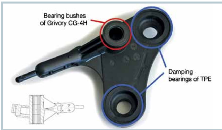
Fig. 2. Bracket for a car windshield washer made from fiberglass-reinforced PPA, with bearing bushes of carbon fiber-reinforced PPA and damping bearings of TPE
