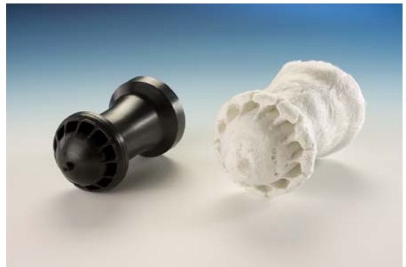
Metal replacement today: Long-fibre reinforced polyamides provide very high strength values and low warpage. To the right, the fibre skeleton of an ashed component.
