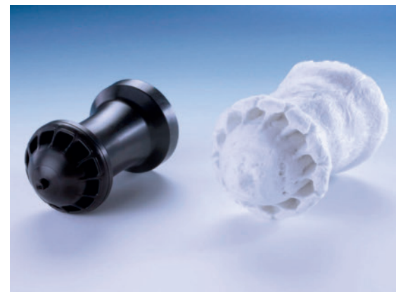
Fig. 1. A three-dimensional fiber network (right) gives semi-crystalline polyamide high-performance properties that are even superior to those of most pressure diecasting alloys
