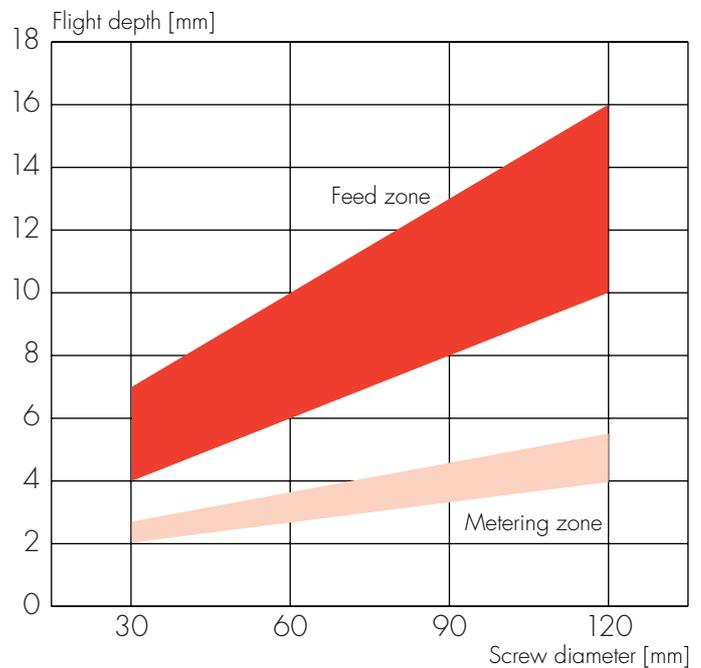
Fig. 18: Recommended flight depths for polyamide screws
