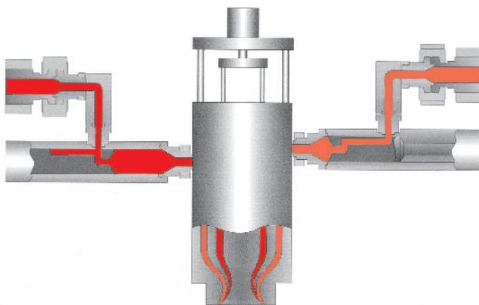
Fig. 15: Sequential blowing head with external melt accumulators
