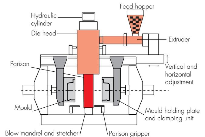
Fig. 11: Components of a blow moulding machine
