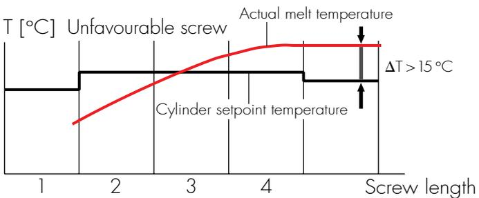
Fig. 17a: Melt temperatures attainable with an unfavourable screw
