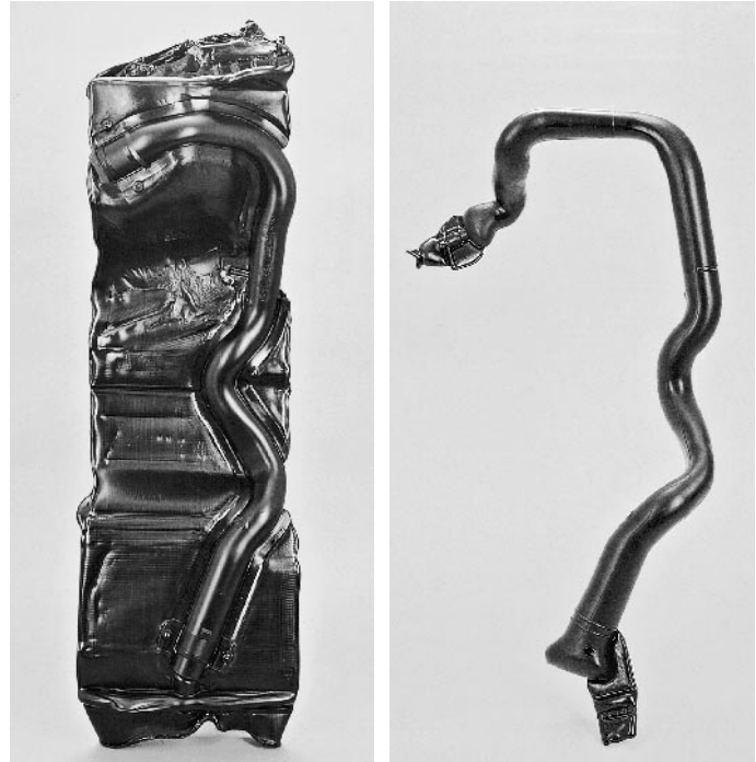
Fig. 14: Blow moulding produced by the conventional process (left) and 3D blow moulding (right).
