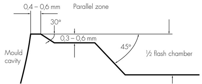
Fig. 21: Recommended pinch-off geometry for polyamide processing
